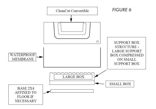
It is important to understand that each tub has variations and modifications may be necessary in the field. For fiberglass and other types of tubs, it may be necessary to adjust the installation of the support boxes based on the framing or support material present on the inside channel of the tub. For example, you may only need to use one of the support box structures based on the height of the bathtub.
